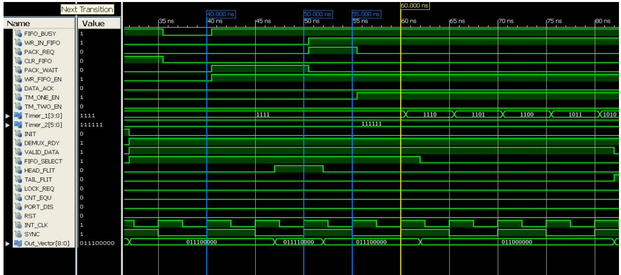
Fig. 6. Start of writing a packet into a queue of the input buffer
